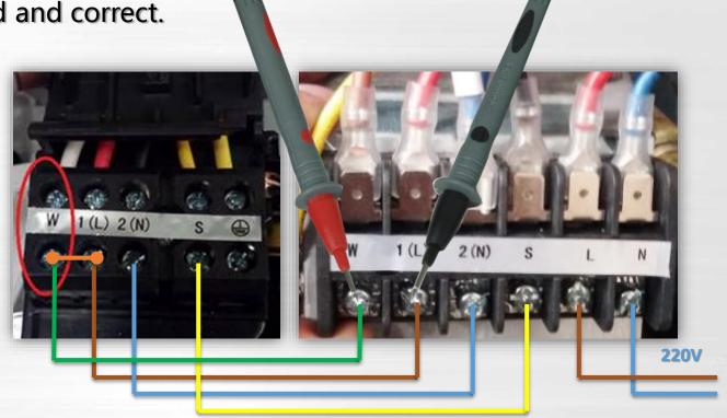
Note: sometimes, it is necessary to test with a temporary cable, because if the cable is bitten, it is likely that the multi-me er indicates continuity by some filament that has been left, but it is not enough for the cable to communicate correctly.
